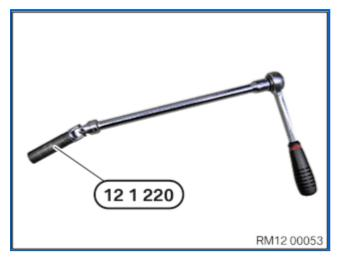
Unscrew spark plugs with special tool <u>12 1 220</u> and with an extension of at least 8° kink.
