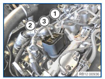
Thread out and install ignition coil (3).
