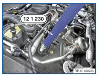
Do not let spark plugs fall into the spark plug shaft. This can lead to a reduction of the electrode gap and so impair the smooth running of the engine, especially in idle mode.
