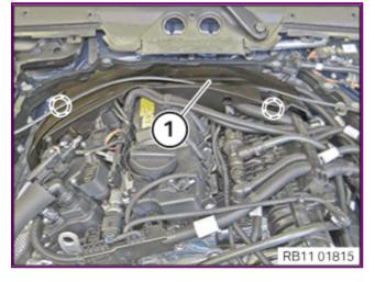
Feed out acoustic cover (1) upwards, out of the guides in the marked area.
