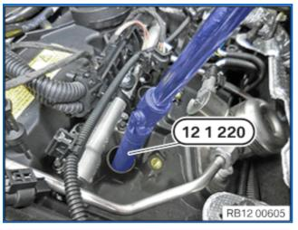
Unscrew spark plugs with special tool <u>12 1 220</u> and an extension with joint.
