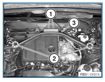
Lever out covers (1) and release screws underneath.
