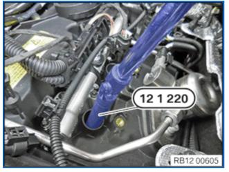
Flexible ratchet extensions must always be used. If rigid mounting tools are used, there is a risk of insulator breakages.
