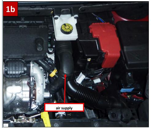
♦ Remove the air supply. This is only clipped.
